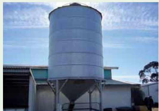
Workplace design – Silos are commonly used to store high volume feed stock instead of handling large numbers of bags.
