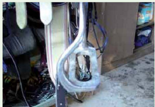
Safety irons used for track work.
