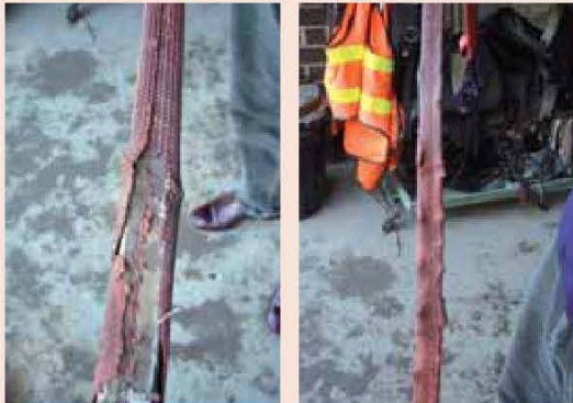
Riding reins – damaged and worn.
