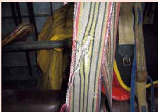
Girth straps – damaged and worn.
