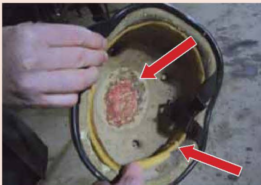
Riding helmet - damaged and well over five years old.
