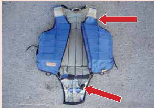
Body protector – damaged with excessive wear.
